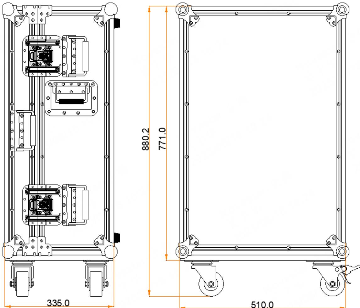
Tolerance:  $\pm 5$  Unit: mm
