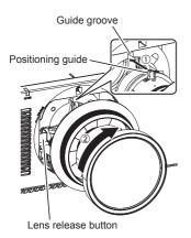
Pass the rear of the zoom lens through the lens mount cover until the lens mount cover is at about the front of the zoom lens.
