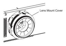
1) Turn the lens mount cover counterclockwise to remove it.
