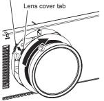
5) Insert the tab on the lens mount cover through the slot on the projector, and turn clockwise to secure lens mount cover.
