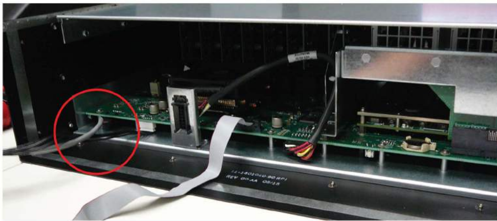
Image 14-35 USB Ext Cable connected to the Motherboard
