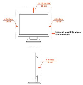
Never install the display set where air-circulation is blocked.
