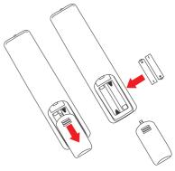
5. Close the battery cover making sure the tabs rest in the corresponding holes and push down the cover until it clicks shut.
